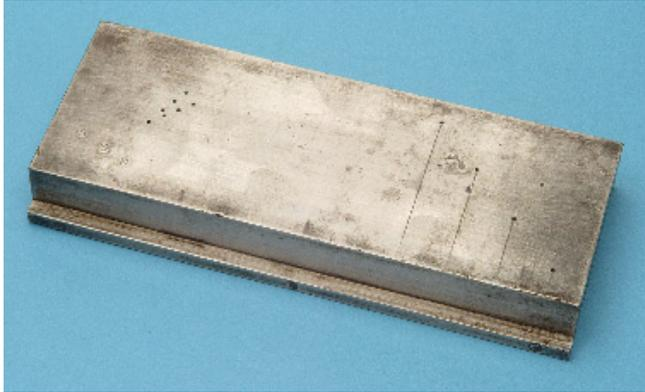
**Figure 14.6 Example of bespoke reference block to check beam characteristics including beam edge resolution and near-zone approximation.**
