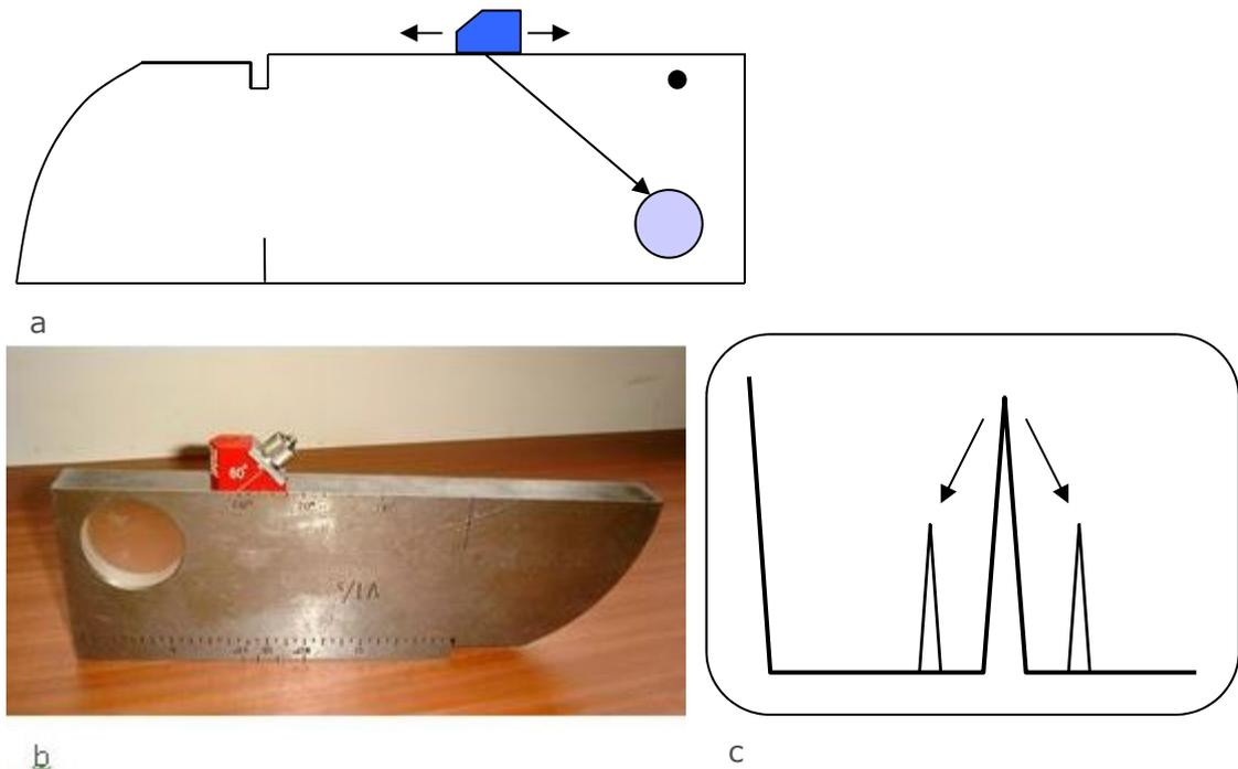
**Figure 12.2 Determination of probe angle:**
