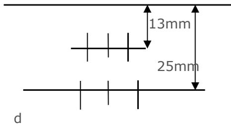
Repeat using the 32mm hole. Join up the points marking the probe centre at 20dB to obtain a beam plot.
