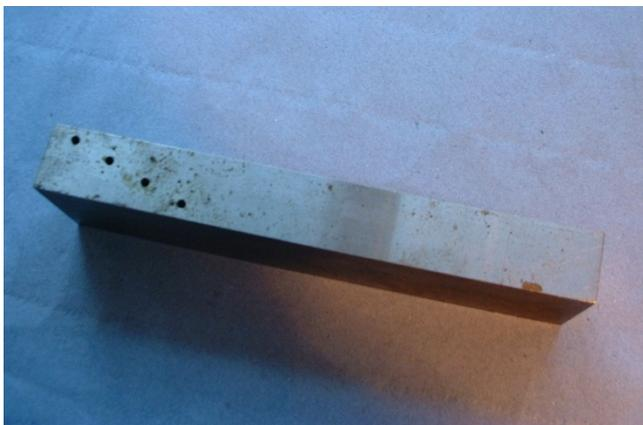
**Figure 15.2 Distance amplitude correction (DAC) reference block.**
