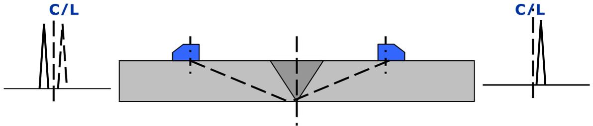
Figure 18.3 Root crack.
