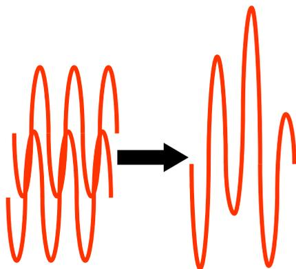
**Figure 5.2 Additive nature of two sound waves interacting.**
