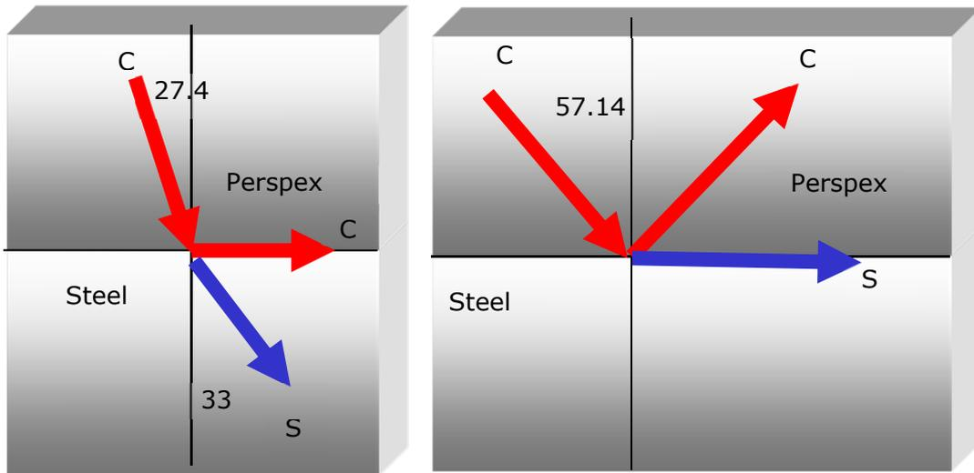
**Figure 8.4(a) First critical angle. (b) Second critical angle.**
