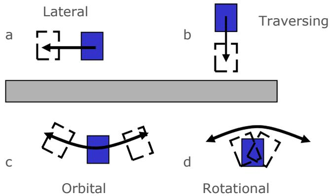
**Figure 17.2 Probe movements to determine echodynamic patterns:**
