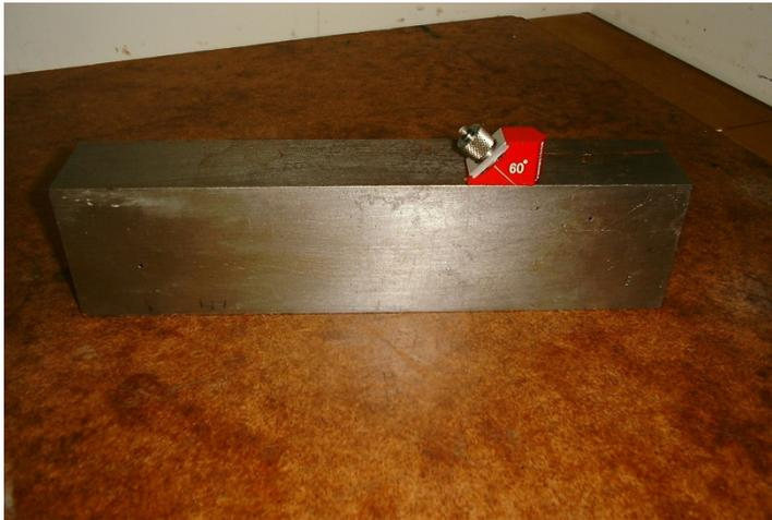
**Figure 15.1 The IOW reference block containing a series of 1.5mm SDH at different depths. A 60° angle probe is shown in position on the block.**
