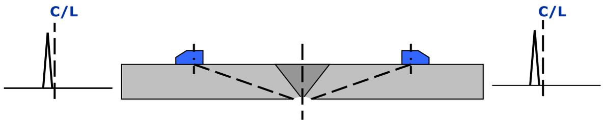
Figure 18.2 Root concavity.
