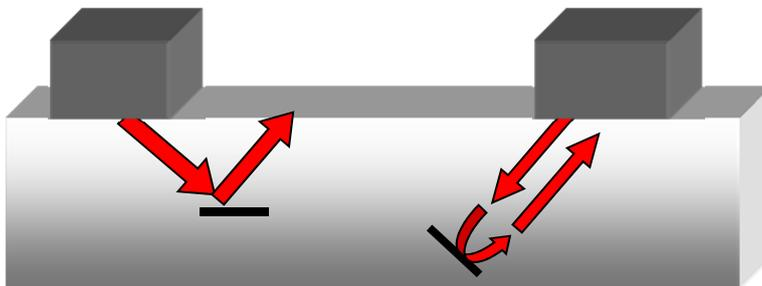
**Figure 10.2 Schematic drawing of the pulse echo technique showing specular reflection from a discontinuity: Shear wave angle probe.**
