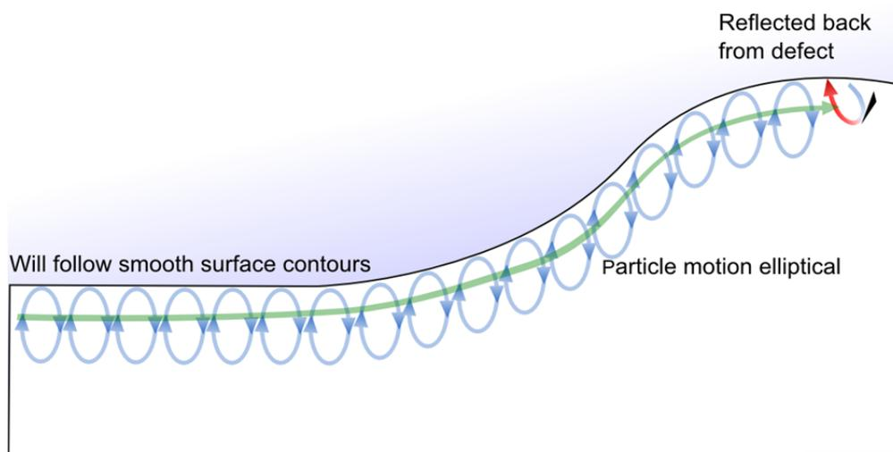
**Figure 2.4 Surface wave propagation.**
