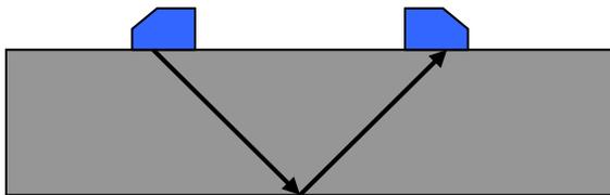
**Figure 15.4 Schematic drawing of the transfer correction method for angle probes.**
