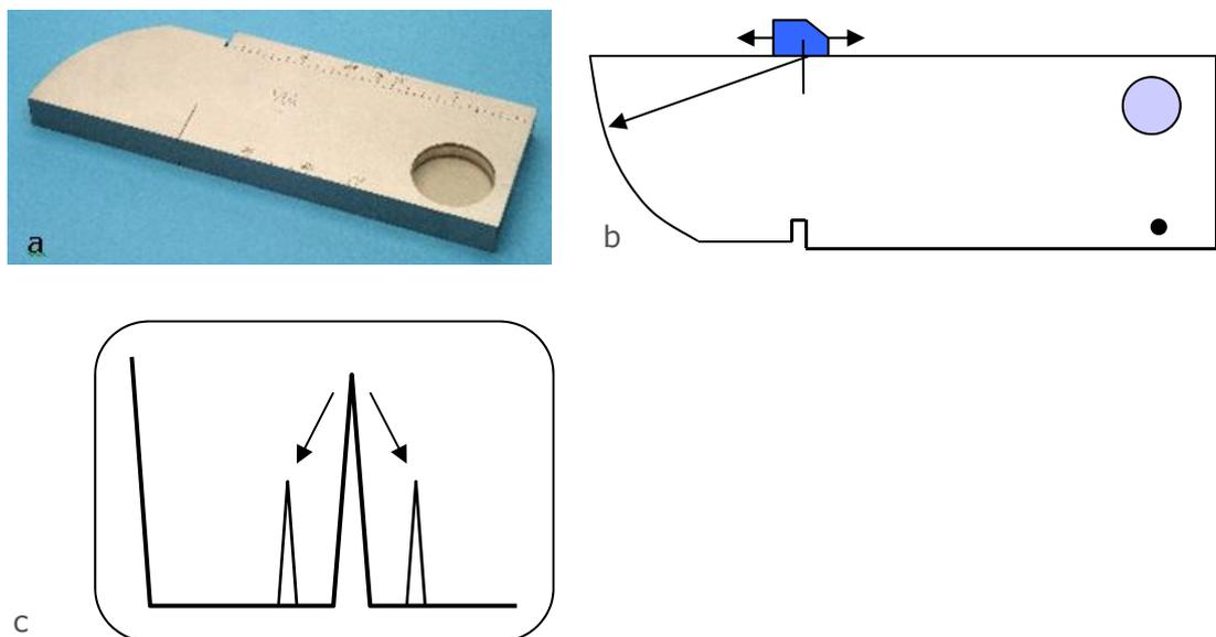
**Figure 12.1 Determination of probe index:**
