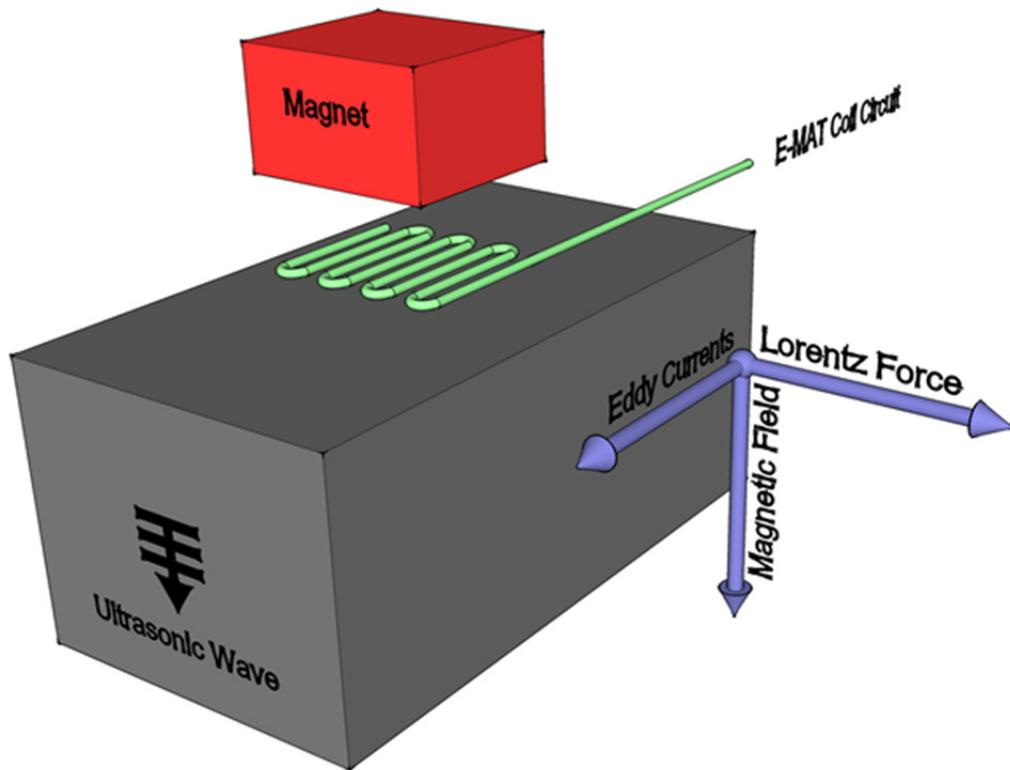
**Figure 3.3 Method of ultrasonic wave generation from an EMAT probe.**
