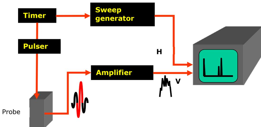
**Figure 11.1 Block diagram of an ultrasonic flaw detector instrument.**
