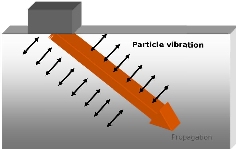
**Figure 2.3 Shear wave propagation.**
