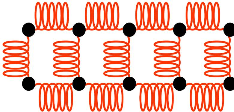
**Figure 2.1 Representation of sound wave propagation using partial mass and microscopic restoring spring forces.**
