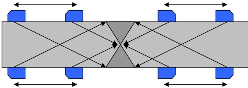
**Figure 21.8 Weld body scan between a ¼ and ½ skip stand-off using 45° and 60° probes.**
