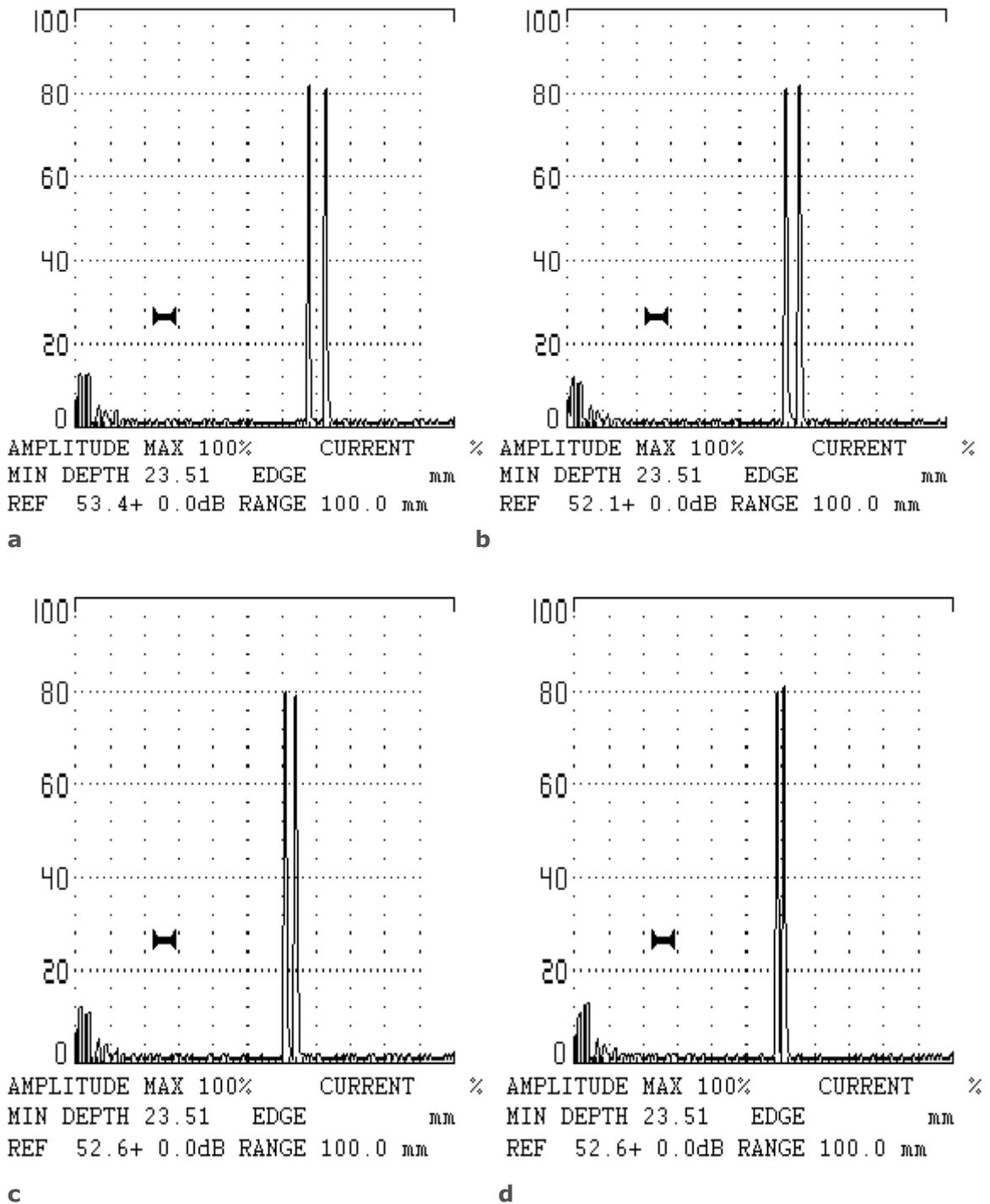
**Figure 16.6 Flaw detector and probe system resolving power (resolution) check to give separate indications of closely situated reflections (note how discontinuities a and b above give clear echo resolution).**
