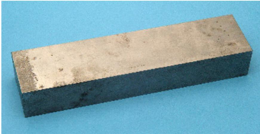
**Figure 14.4 IOW reference block with 1.5mm side-drilled holes at different depths.**
