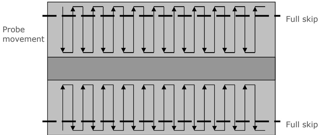
**Figure 21.2 Parent material comparison probe scan.**
