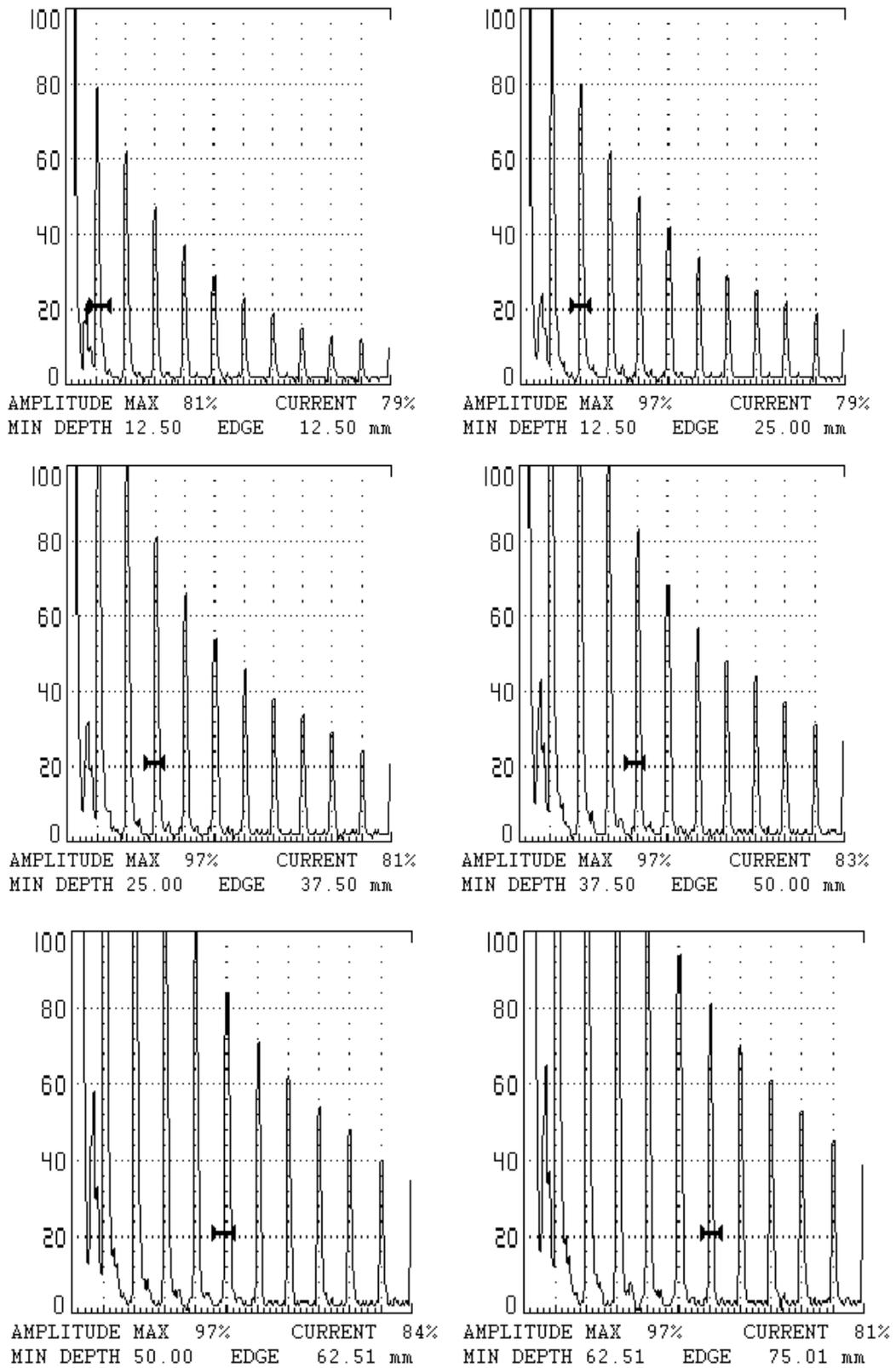
**Figure 16.2 'A' scan (echo amplitude at approximately 80% vs depth distance) presentations.**
