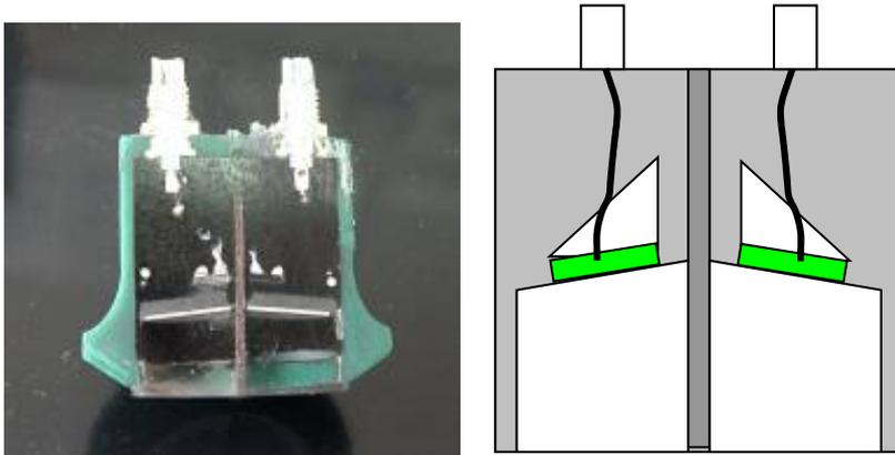
**Figure 9.4 Twin crystal probe: Photograph and schematic drawing.**
