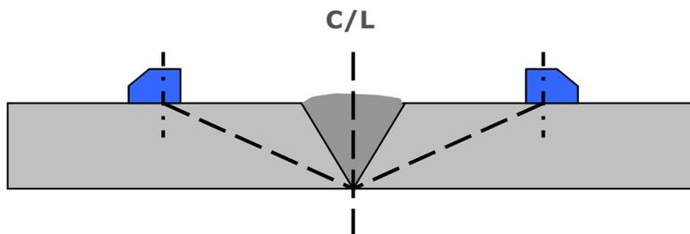
**Figure 21.1 Weld root detection.**
