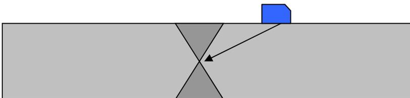
**Figure 21.7 Double V weld root examination from 1/4 skip.**
