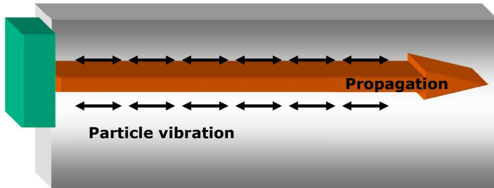
**Figure 2.2 Compression wave propagation.**
