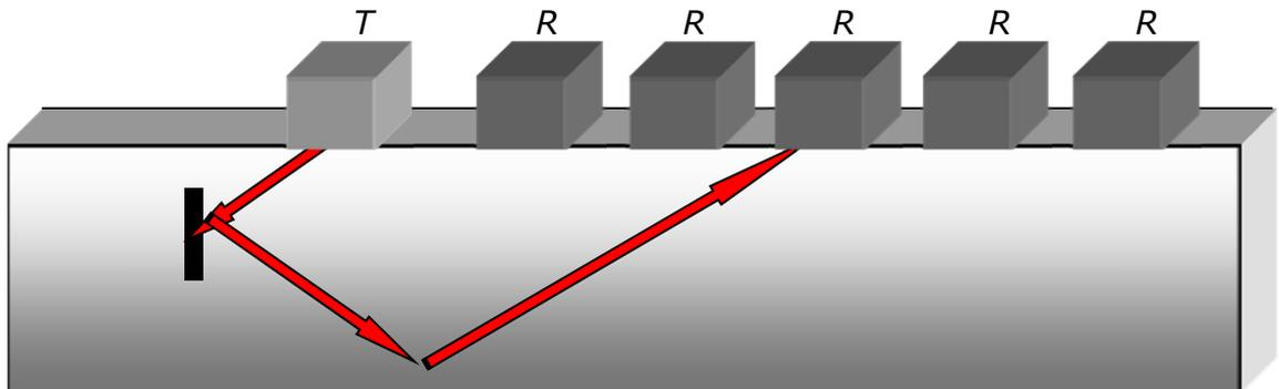
Figure 10.4 Tandem scanning (T=Transmitter, R=Receiver).
