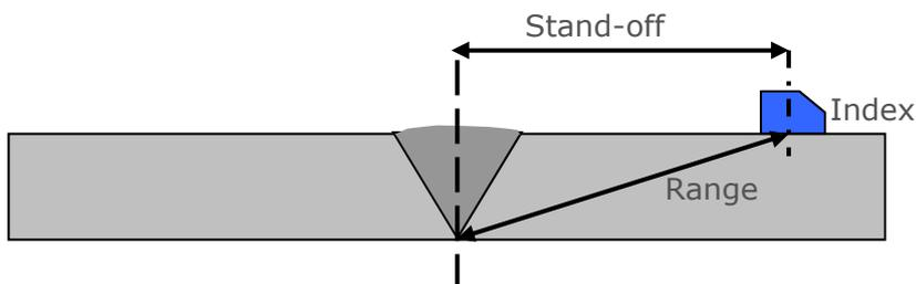
**Figure 21.3 Root Scan using an angle probe at a fixed 'stand-off'**
