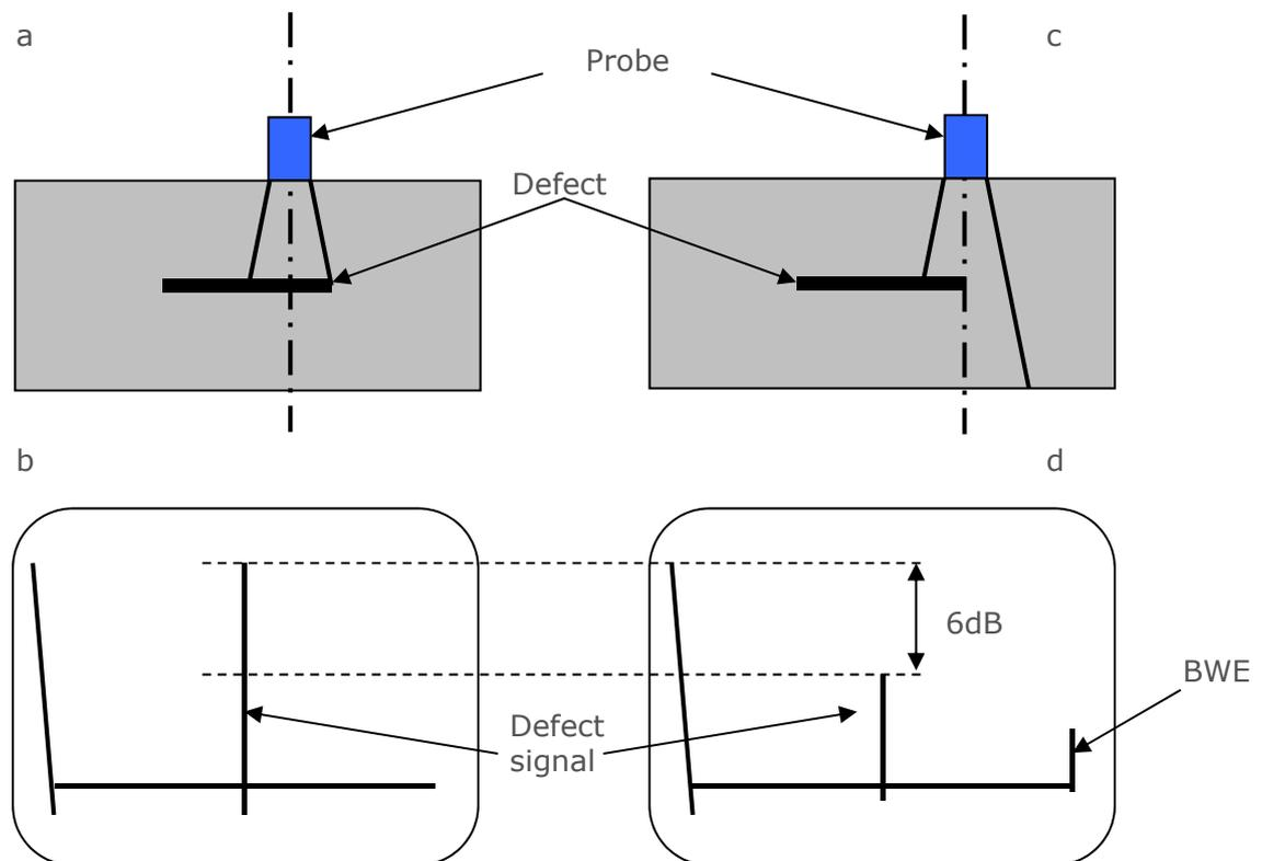
**Figure 14.1: 6dB drop sizing:**
