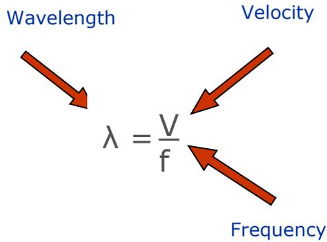
**Figure 1.3 Wavelength, Velocity and Frequency relationships.**
