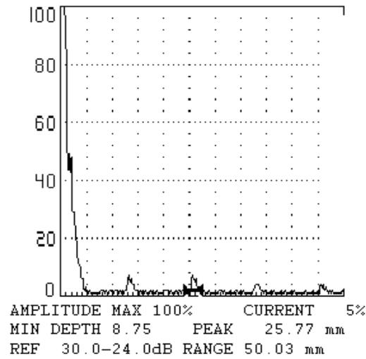
**Figure 16.4 Amplifier and gain control checks at 0db to 24db.**
