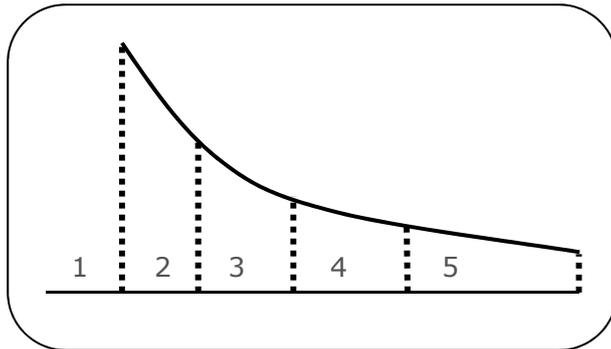
**Figure 15.3 DAC construction from a series of reflector SDHs to cover the thickness range of the test component.**
