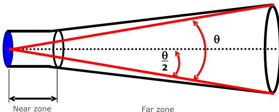
**Figure 5.6 Beam spread.**
