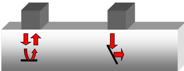
**Figure 10.1 Schematic drawing of the pulse echo technique showing specular reflection from a discontinuity: Normal compression probe.**
