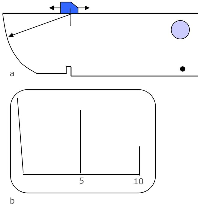
**Figure 12.3: Calibration of the time base (range) of the flaw detector:**
