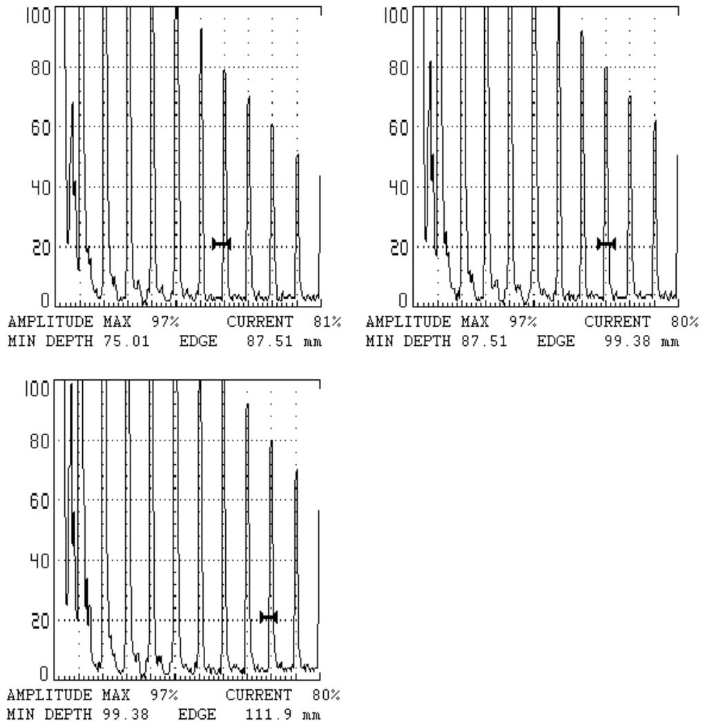
**Figure 16.3 'A' scan presentations showing respective echoes set at 80% FSH.**
