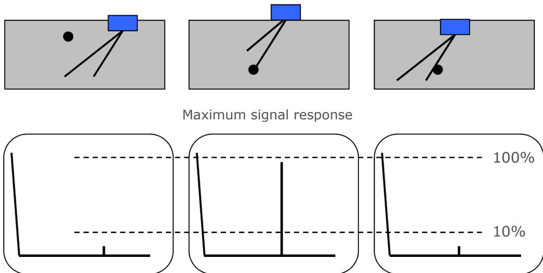
**Figure 14.5 Angle beam plot construction.**
