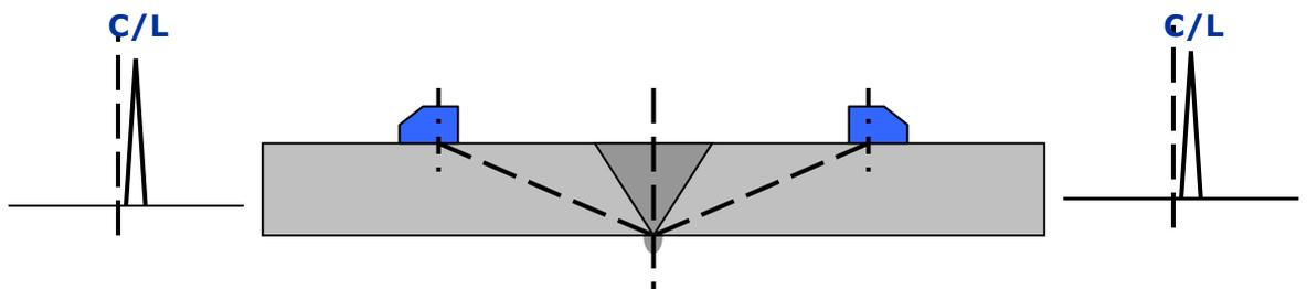
Figure 18.1 Excess penetration.
