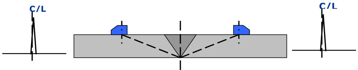
Figure 18.4 Lack of root fusion.
