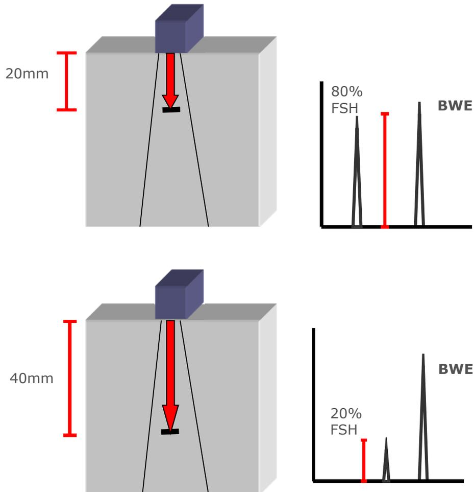
Figure 6.3 Law of the small reflector (ie smaller than the beam width).
