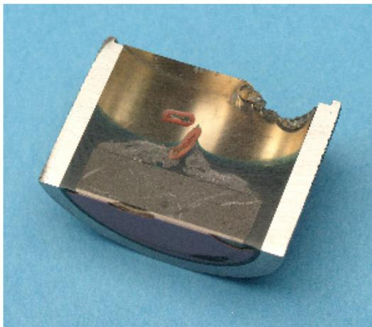
**Figure 9.2 Compression wave probe: Cross section.**
