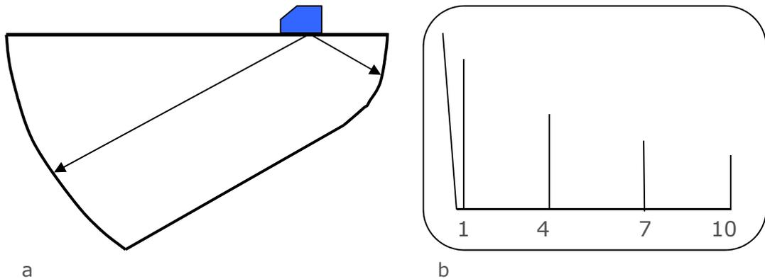
**Figure 12.6 Block No 2 Calibration for 250mm range:**
