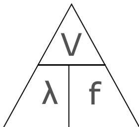
If we want to work out wavelength we cover the wavelength symbol - this leaves  $V$  over  $f$ . If we need to find the velocity, cover the  $V$  which gives us  $\lambda \times f$ . Covering the frequency ( $f$ ) will leave  $V$  over  $\lambda$ .
