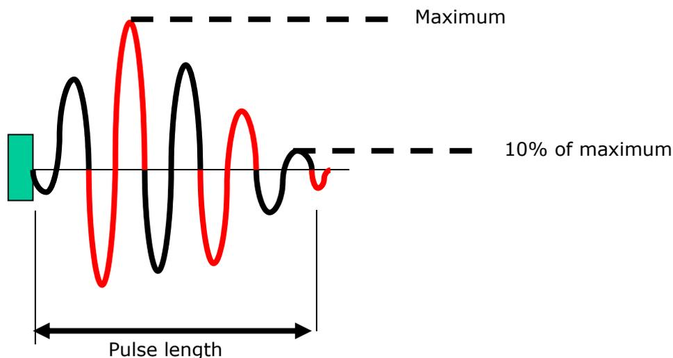
**Figure 4.1 Ultrasonic pulse.**
