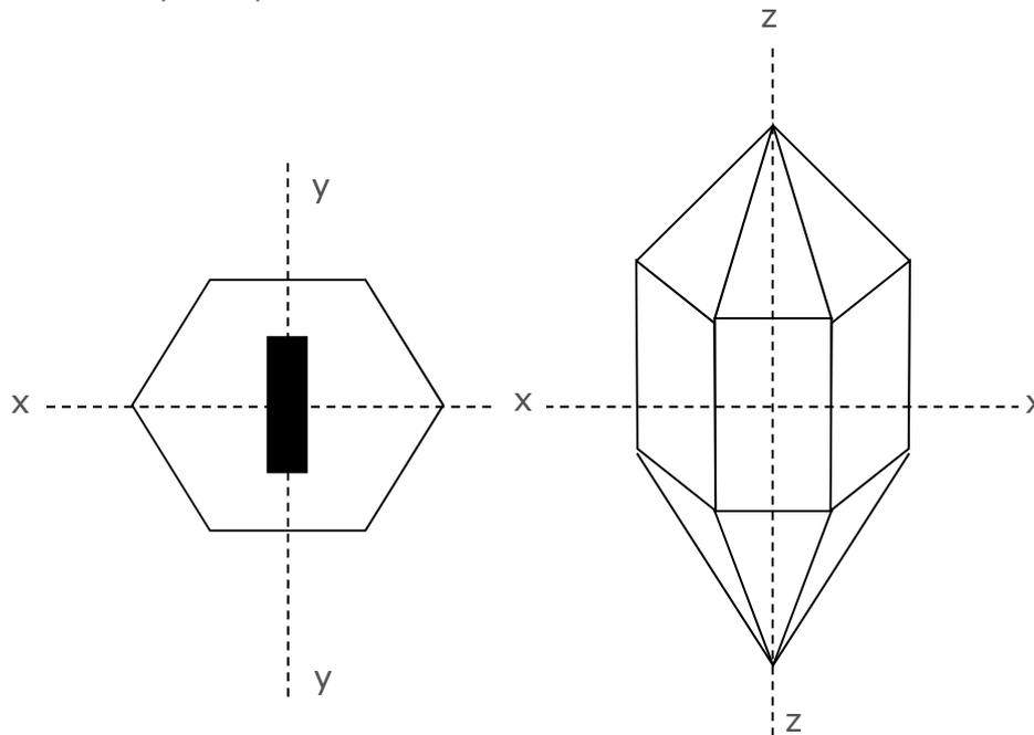
**Figure 3.2 X-cut quartz crystal.**
