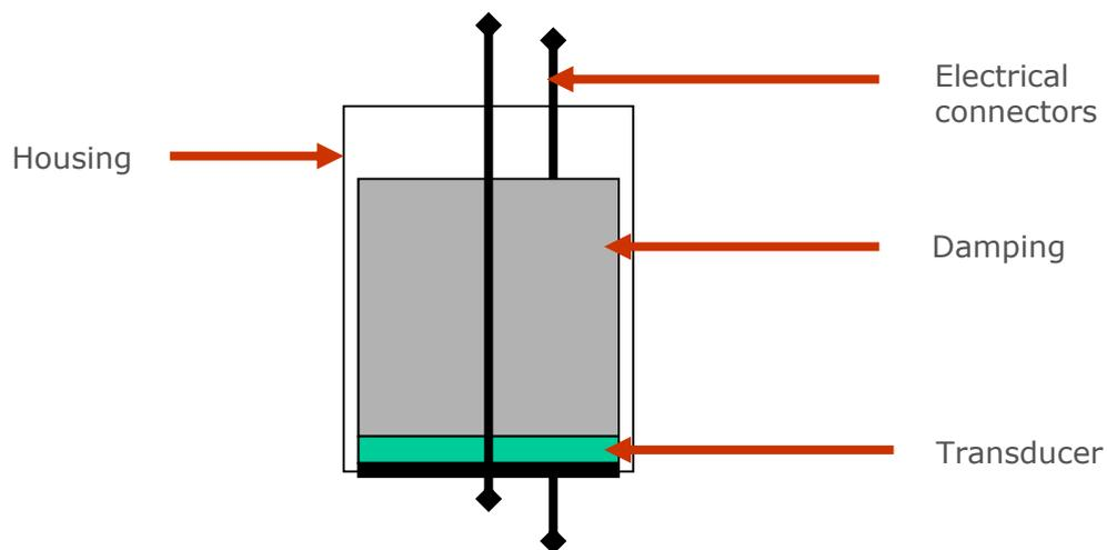
**Figure 9.1 Compression wave probe: Schematic drawing.**
