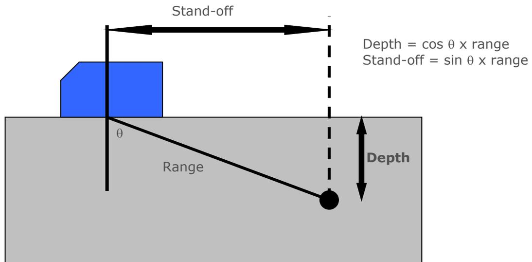
**Figure 13.1 Reflector depth and probe stand-off as a function of probe angle.**
