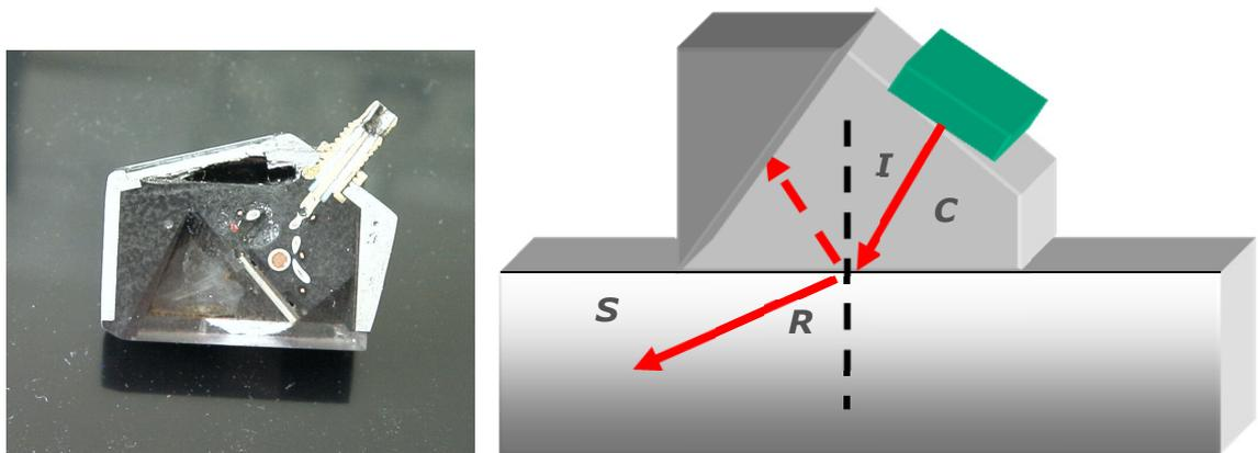
**Figure 9.3 Angle probe: Photograph and schematic drawing.**
