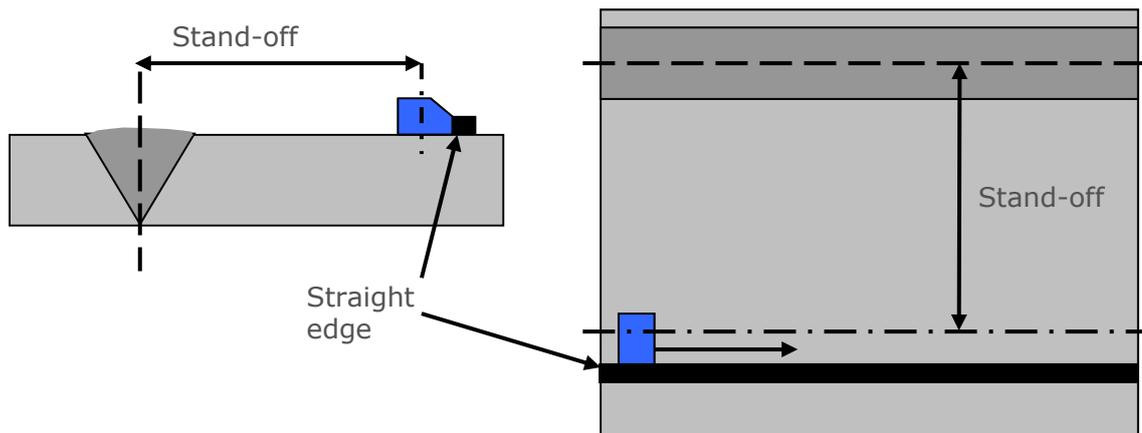
**Figure 21.4 Fixed 'stand-off' scan using a straight edge.**
