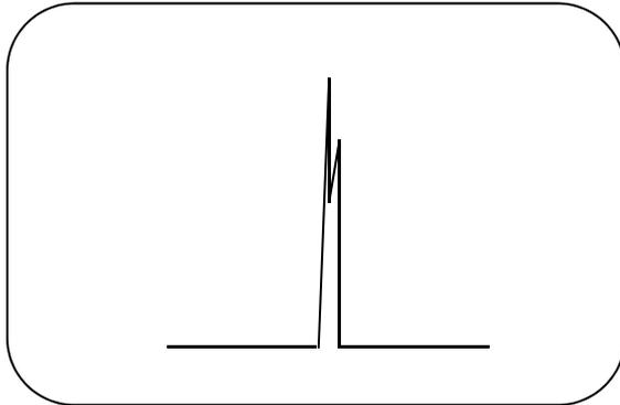
**Figure 19.5 Linear inclusion (slag).**
