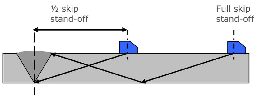
**Figure 21.5 Angle probe raster scanning from the weld cap edge to the full skip position.**
