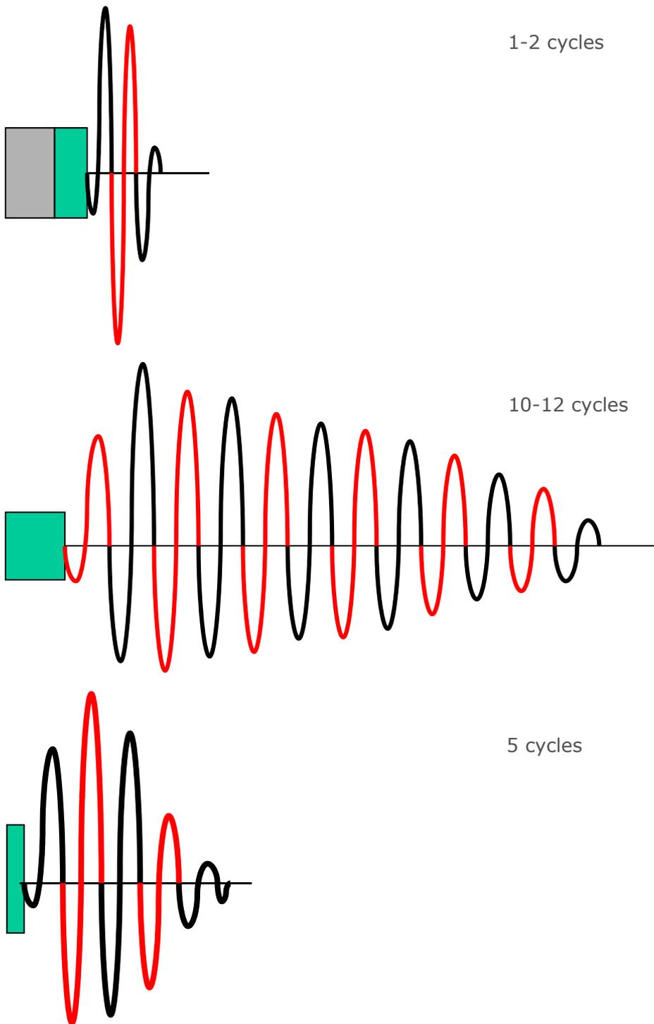
**Figure 4.2 Pulse lengths.**
