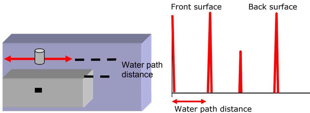
Figure 10.6 Immersion scanning.
