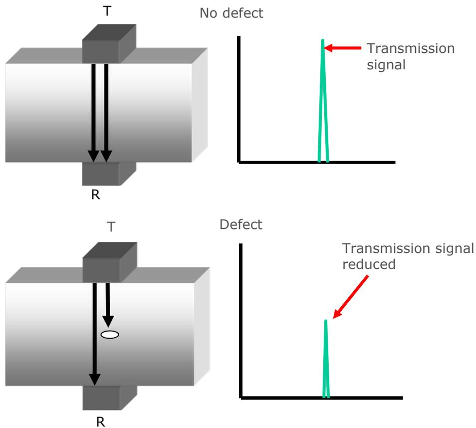
**Figure 10.3 Through-transmission.**
