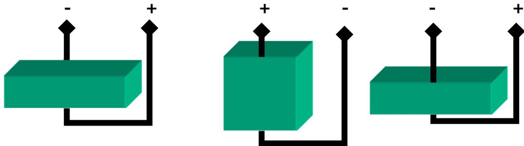
**Figure 3.1 Illustration of the piezo-electric effect showing the effect of an applied voltage on a crystal.**
