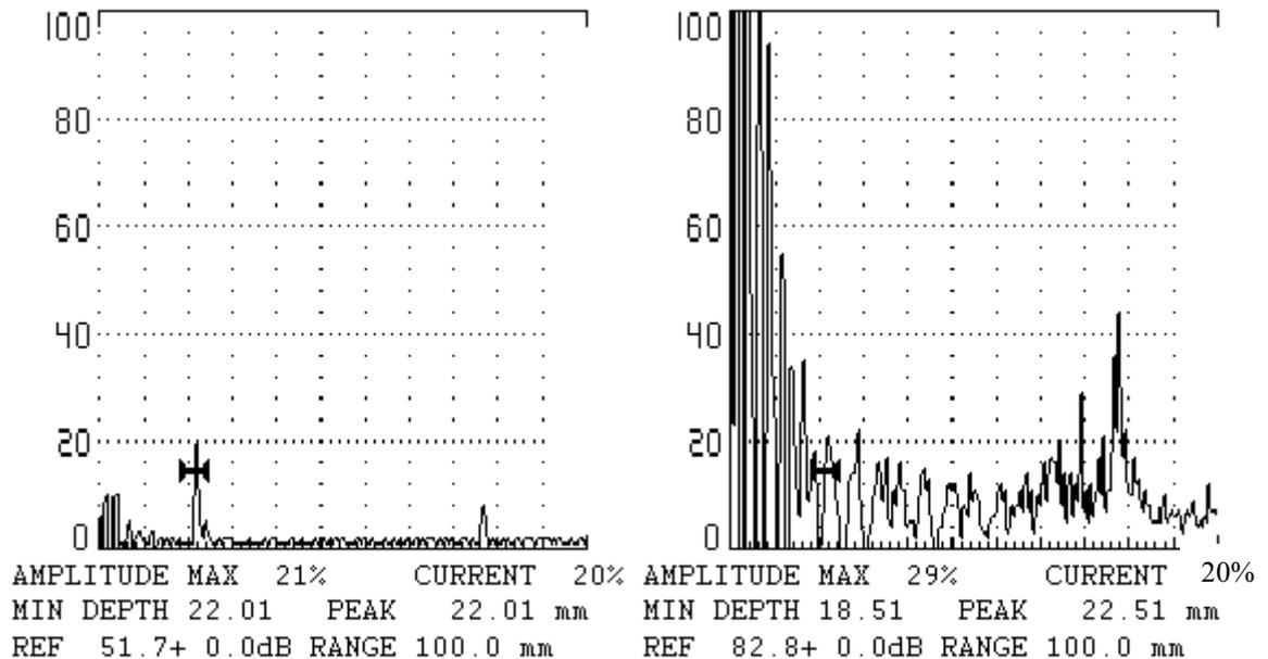
**Figure 16.5 Sensitivity and signal-to-noise ratio (SNR) check.**
