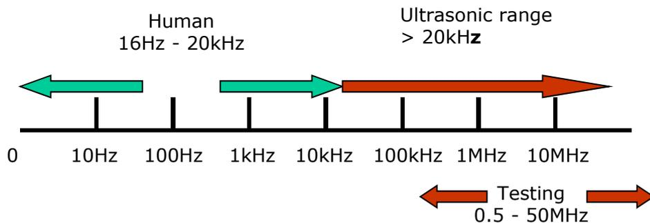
**Figure 1.2 The sound spectrum.**
