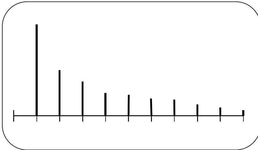
**Figure 16.1 'A' scan flow detector showing signal amplitude vs distance (transit time) for linearity of time base checks.**
