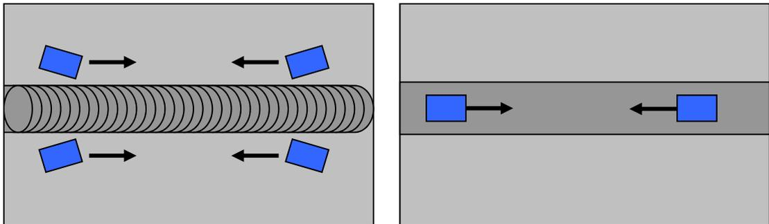
**Figure 21.6 Shear wave angle probe scan to detect transverse defects.**
