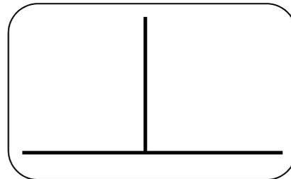
Move the probe to one side until the signal drops to 10% FSH (-20dB) and mark the centre of the probe on the side of the block.
