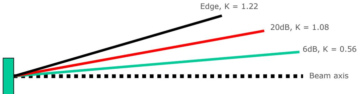
**Figure 5.7 K values for the beam edge.**
