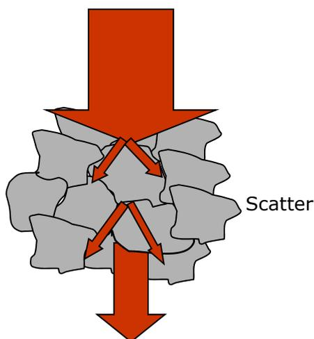
**Figure 6.1 Scatter of the ultrasonic beam at grain boundaries.**
