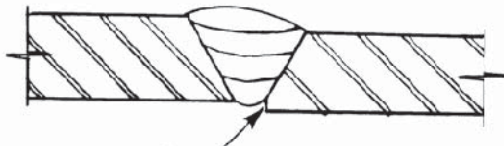
Incomplete filling at root on one side only
