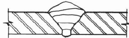
(g) Excess External Reinforcement
